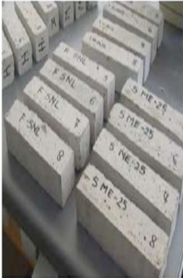
Condition of the plaster samples after examination on resistance to salt crystallization
